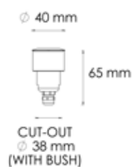
L0217 COURTESY LIGHT \varnothing mm 40 1 W
